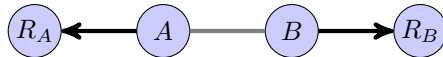
Figure 5.21: The exposed terminal problem: senders A and B could send to their respective recipients R_A and R_B simultaneously, but believe it would cause collisions due to carrier sensing.
