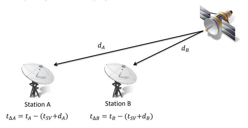
$$t_{\Delta} = t_{\Delta B} - t_{\Delta A} = t_B - (t_{SV} + d_B) - t_A + (t_{SV} + d_A) = t_B - t_A + d_A - d_B$$
