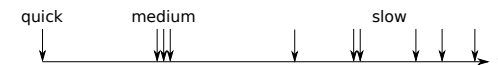
■ Figure 2 Waiting time of nodes in different states: A quick node creates a block instantly when seeing a new transaction. A medium node waits long enough to ensure not to compete with a quick node. A slow node waits long enough to ensure to compete neither with a quick nor a medium node. The figure represents a situation with one quick, three medium, and some slow nodes.
