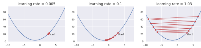
Figure 5.28: Gradient descent with different learning rates for finding the minimum of a quadratic function. On the (left) the learning rate is very low so convergence is slow and on the (right) the learning rate is too high so gradient descent diverges.
