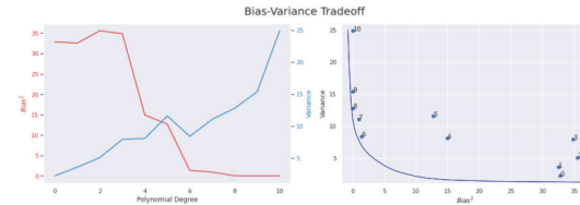
Figure 5.22: Fitting polynomials of increasing degree to the cosine function within the range [-5, 5] . On the left we see that as the degree (complexity) of the model increases, the bias decreases and the variance increases. The plot on the right shows the bias variance tradeoff frontier.
