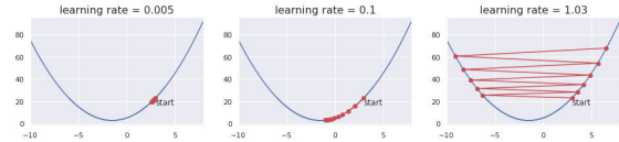
Figure 5.28: Gradient descent with different learning rates for finding the minimum of a quadratic loss function. On the (left) the learning rate is very low so convergence is slow and on the (right) the learning rate is too high so gradient descent diverges.
